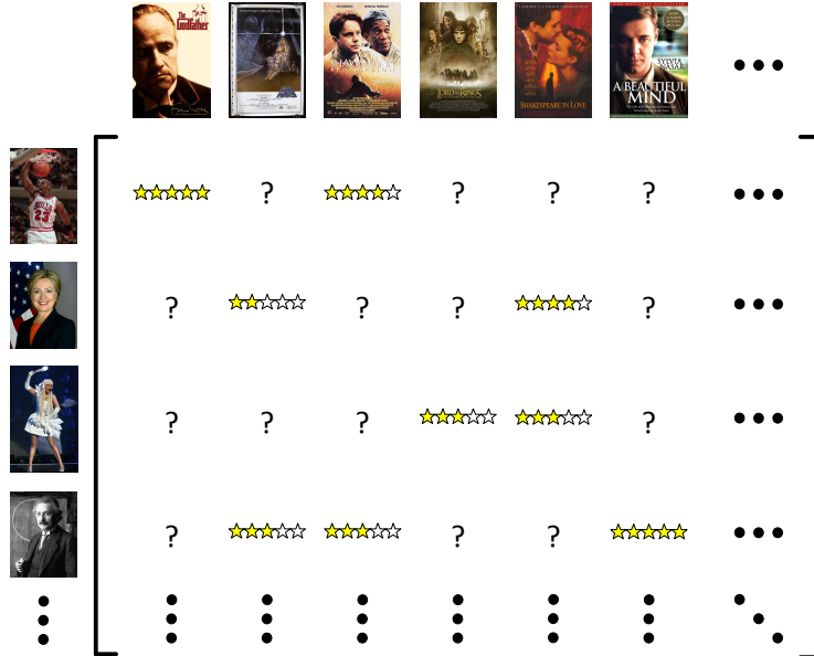
Figure 1: A depiction of the Netflix challenge in matrix form. Each row corresponds to a user that ranks a subset of the movies, which correspond to the columns. The figure is due to Mahdi Soltanolkotabi.
