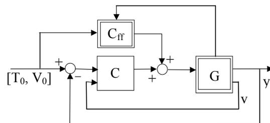
Fig. 6. Control strategy with additive measures and feedforward signals
