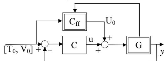
Fig. 4. Control strategy with feedforward signals
