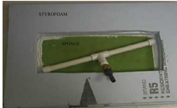
Figure 2: The diffuser allows the freshwater to be poured slowly so that a sharp interface is created between the two layers.
