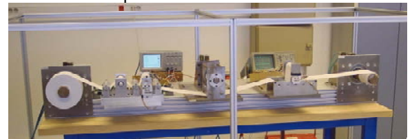
Fig. 1. Experimental setup with 3 brushless motors and 2 load cells
